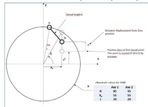
Fig.4: OSM deviation working principle
